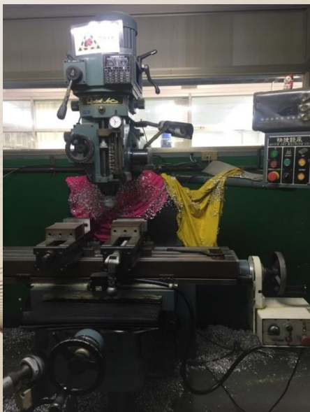
Quick Jet QJM-QB-VA Main Spindle : 75~3600RPM
